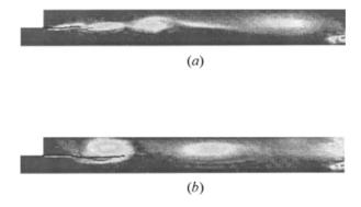
Figure 7.9 Vorticity distribution and droplet locations for microexploding droplets of initial diameter 35  $\mu$ m (a) and 50  $\mu$ m (b)
