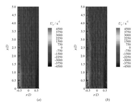
**Figure 18.7** Time-averaged strain  $U_r$  and velocity field (a) and instantaneous strain and velocity field (b) of the premixed flame for  $-U_2/U_1 = 0.022$ . The scale of the velocity vector length is 7.2 m/s per 1 mm
