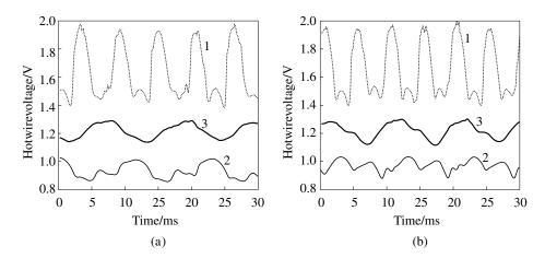
**Figure 6.6** Velocity—time traces of the main air jet at the centerline (1), fuel jet (2), and external air entrainment (3), measured at the jet exit plane, for low-soot forcing (a) and high-soot forcing (b)
