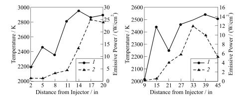
Figure 8.4 Measured temperature and radiation intensity distributions for the O<sub>2</sub>/Ar oxidizer test in 24-inch long combustor. 1 — temperature, 2 — power, 425–800 nm
