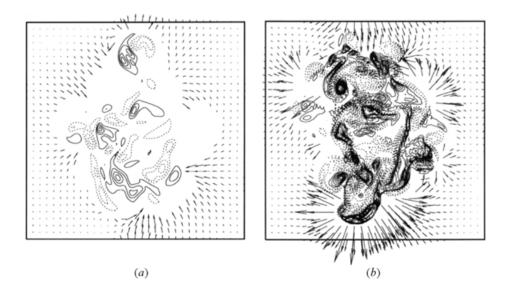
**Figure 11.5** Comparison of computed entraining velocity fields at the widest transverse sections of the (a) unheated and (b) heated jet at time t=35. The contours of streamwise vorticity, at intervals of 0.5, are shown using solid lines for positive values, and dotted lines for negative values. Contour for level 0 is not shown
