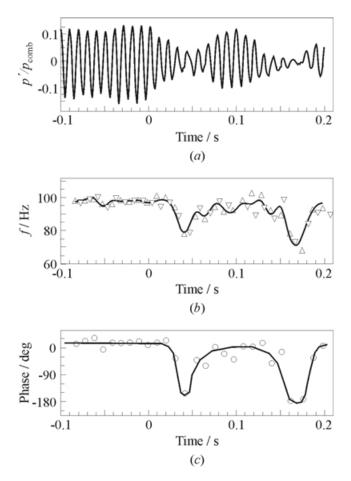
**Figure 21.15** Transient system response to onset of control at time t = 0 in Case 3A: (a) measured amplitude, (b) apparent frequency of pressure oscillations, and (c) fuel injection phase based on the controller frequency response
