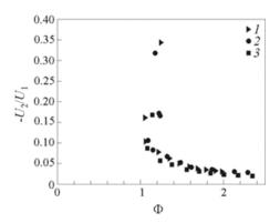
**Figure 18.5** Variation of velocity ratio with equivalence ratio for different collar dimensions with  $Q_2 = 5.5 \cdot 10^{-5}$  m<sup>3</sup>/s: 1 - W/D = 0.21 (U = 0.71 m/s); 2 - 0.23 (U = 0.60 m/s); and 3 - 0.31 (U = 0.41 m/s)
