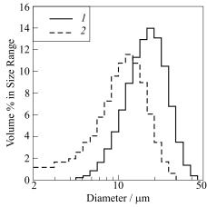
Figure 8.8 Particle size distribution of fuel and unburned fraction in products from  $\rm H_2O$  oxidizer test: 1 — fuel, 2 — products
