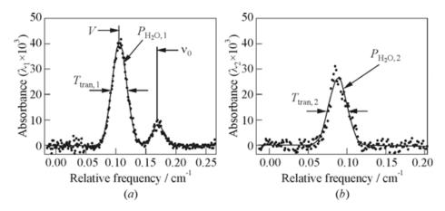
**Figure 24.15** Single-sweep data traces of H<sub>2</sub>O absorption recorded in a hypersonic flow with an enthalpy of 10 MJ/kg. The panels shows the absorbance (as a function of laser frequency, cm<sup>-1</sup>) near 1.400  $\mu$ m (a) and 1.395  $\mu$ m (b) recorded simultaneously.  $V=4630\pm50$  m/s;  $T_{\rm tran,1}=561\pm15$  K;  $P_{\rm H_2O,1}=0.43\pm0.03$  Torr;  $T_{\rm tran,2}=544\pm35$  K; and  $P_{\rm H_2O,2}=0.45\pm0.06$  Torr
