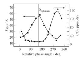
**Figure 24.11** Variation of  $T_{\rm RMS}$  (left axis) values measured at port 1 (x/d=4) and CO concentration (right axis) of gases sampled from port 4 (x/d=14) with relative phase angle between primary and secondary air driving in the 50-kilowatt forced combustor at China Lake
