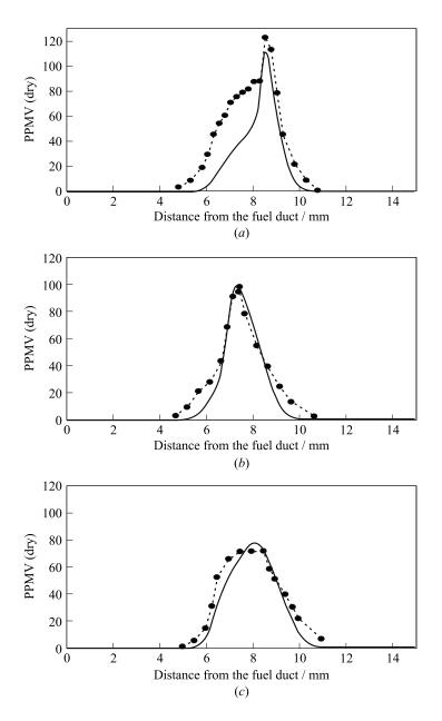
**Figure 27.3** Measurements and predictions of mole fractions of NO as a function of distance from the fuel duct for diffusion (a) and partially premixed opposed flow flames with  $\Phi_B=2.2~(b)$  and 1.42~(c),  $T_{\rm air}=560~{\rm K}$  and  $T_{\rm fuel}=321~{\rm K}$ ,  $V_{\rm air}=70,60$ , and  $50~{\rm cm/s}$ ,  $V_{\rm fuel}=70~{\rm cm/s}$ , distance between ducts  $1.5~{\rm cm}$
