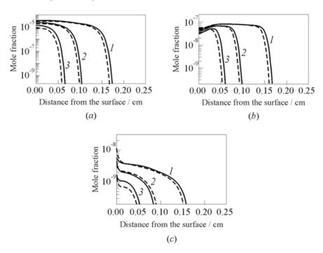
**Figure 26.8** Profiles of NO (a), N<sub>2</sub>O (b), and NO<sub>2</sub> (c), corresponding to Fig. 26.7:  $1-\alpha=3000~{\rm s}^{-1};~2-5000;$  and  $3-8000~{\rm s}^{-1}$
