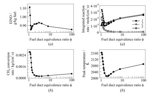
**Figure 27.4** Predictions of EINO (a) and CH<sub>4</sub> consumption rate (b) as a function of fuel duct equivalence ratio  $\Phi_B$  for opposed flow flames with  $T_{\rm air}=560$  K and  $T_{\rm fuel}=300$  K;  $V_{\rm air}=70$  cm/s,  $V_{\rm fuel}=70$  cm/s, distance between ducts 1.5 cm
