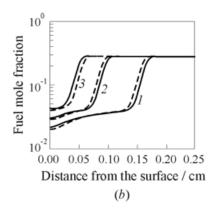
**Figure 26.7** Profiles of temperature (a) and fuel (b) for surface temperatures of 500 K (dashed curves) and 1000 K (solid curves) for a 28% inlet H<sub>2</sub>-air mixture. The conditions of pressure and inlet temperature are the same as in Fig. 26.4. 1 —  $\alpha = 3000 \text{ s}^{-1}$ ; 2 — 5000; and 3 — 8000 s<sup>-1</sup>
