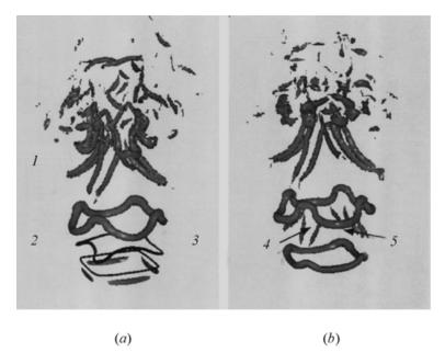
**Figure 13.3** Instantaneous isosurfaces of the vorticity magnitude for the square jet [9] at two times  $t_1$  (a) and  $t_2$  (b). 1 — hairpin rib pairs, 2 — vortex rings, 3 — vortex lines, 4 — flow ejection, and 5 — vortex-ring flattening
