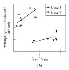
**Figure 29.14** Change in flame lift-off height as a function of (a) excitation frequency and (b) Damköhler number
