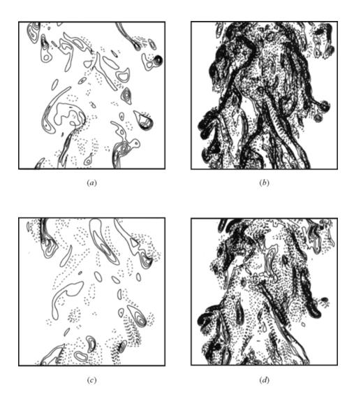
**Figure 11.1** Streamwise sections (in the yz-plane passing through the axis of the jet) of different components of vorticity in the unheated (a), (c) and heated (b), (d) jets at time t=35; (a), (b) — azimuthal vorticity, (c), (d) — streamwise vorticity. Negative contours are shown using dotted lines in steps of -0.5 starting from -0.5, while positive contours are in solid lines in steps of 0.5 starting from 0.5
