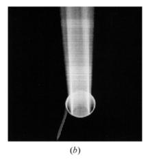
**Figure 18.4** Propane–air premixed flame attached to suction collar rim for  $-U_2/U_1 = 0.0$  (a), and to nozzle exit for  $-U_2/U_1 = 0.022$  (b)
