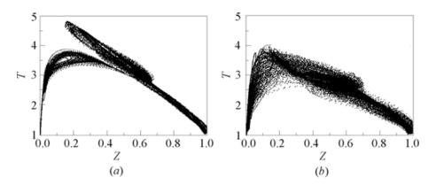
**Figure 10.6** Instantaneous scatter plot of nondimensional temperature vs. mixture fraction: (a) without radiation; (b) with radiation
