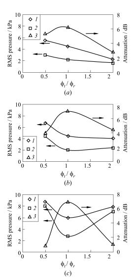
**Figure 19.9** Influence of unpremixedness on control; flow arrangement with swirl; Sw = 0.60;  $U_m = 17$  m/s;  $U_a = 60$  m/s; Re<sub>s</sub> = 56,000;  $\phi_0 = 0.73$ ; (a) 5% of total fuel oscillated, mean equivalence ratio of axial jet,  $\phi_a = 0.73$ ; (b) 7%,  $\phi_a = 1.1$ ; (c) 11%,  $\phi_a = 1.73$ ; 1 — without control; 2 — with control; and 3 — attenuation
