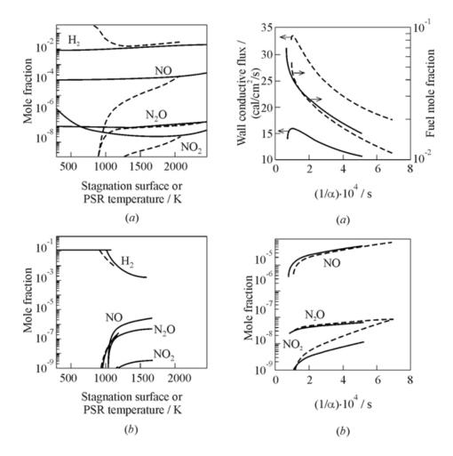
Figure 26.5 Surface mole fractions of fuel and  $NO_x$  as functions of stagnation surface (solid curves) and PSR temperature (dashed curves), for 28% inlet  $H_2$  in air (a) and 12% inlet  $H_2$  in air (b). The maximum temperature indicates adiabatic operation. The conditions are the same as in Fig. 26.4
