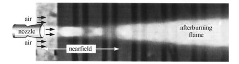
Figure 29.1 Near field of supersonic afterburning plume
