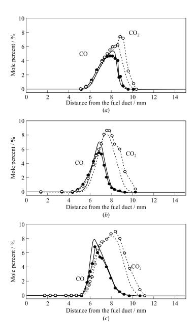
**Figure 27.2** Measurements and predictions of mole fractions of CO<sub>2</sub> and CO as a function of distance from the fuel duct for diffusion (a) and partially premixed opposed flow flames with  $\Phi_B=2.2~(b)$  and 1.42 (c),  $T_{\rm air}=560~{\rm K}$  and  $T_{\rm fuel}=321~{\rm K},\,V_{\rm air}=70,$ 60, and 50 cm/s,  $V_{\rm fuel}=70~{\rm cm/s},\,{\rm distance}$  between ducts = 1.5 cm
