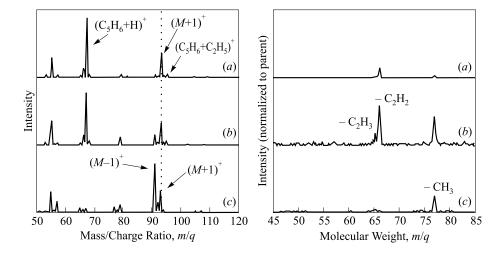
Representative CI mass Figure with flow tube temperature: (a) 973 K; isomers, (b) 573 K; and (c) 298 K
