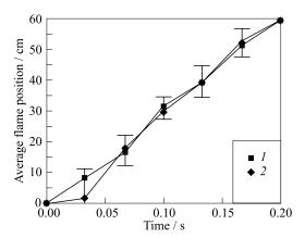
**Figure 15.2** The ensemble-averaged absolute flame position in the TC apparatus, measured from the top of the TC annulus, plotted vs. absolute time (measured from the time of ignition) for  $\phi = 1.1$  and Re<sub>ave</sub> = 7500: 1 — left; 2 — right
