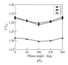
**Figure 20.9** Centerline temperature vs. phase angle,  $N_S = 0.3$  (configuration 1): (a) r/R = 0; (b) 0.67. 1 - x/D = 0.16; 2 - 0.34; and 3 - 0.67
