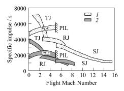
Figure 30.5 Comparison of specific impulse and flight Mach number for hydrogen (1) and hydrocarbons (2). PDE performance estimated using ASI Performance deck; turbojet, ramjet, and scramjet performance levels reflect well-designed systems for man-rated thrust classes. TJ — turbojets; RJ — ramjets; SJ — scramjets; PDE — pulse detonation engines; PIL — preignition limit [12]
