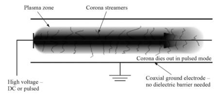
Figure 1.3 Schematic of corona reactor for NO reduction [10]
