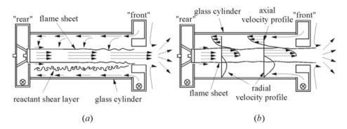
Figure 17.3 (a) Cross-sectional view of the Countercurrent Swirl Combustor; (b) anticipated velocity profiles within the combustor
