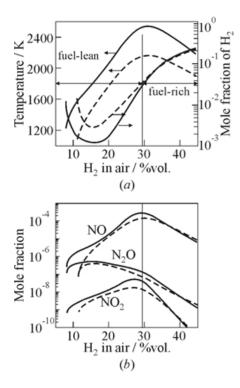
Figure 26.4 Surface temperature and surface fuel mole fraction (a), and  $NO_x$  (b) as functions of inlet composition, along the adiabatic curve, for the stagnation reactor (solid curves) and the PSR (dashed curves). The fuel-lean and fuel-rich regions are indicated. The conditions are pressure of 1 atm, inlet temperature of 25 °C, a strain rate of 1000 s<sup>-1</sup> (stagnation reactor), and a residence time of 1 ms (PSR)
