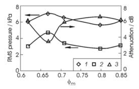
**Figure 19.5** Active control by oscillation of fuel in main flow; annular flow arrangement;  $U_m = U_p = 7.5 \text{ m/s}$ ; Re<sub>m</sub> = 40,000; 1 — without control; 2 — with control; and 3 — attenuation
