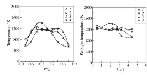
**Figure 28.2** Gas temperature profiles at 2.2 pipe diameters downstream of the nozzle ( $Q_{\rm in}=13.2$  kW,  $\phi=0.237,\ t=25.4$  mm, p=8 ppcm):  $1-L/D=\infty;$   $2-1.5;\ 3-1.1;$  and 4-0.7
