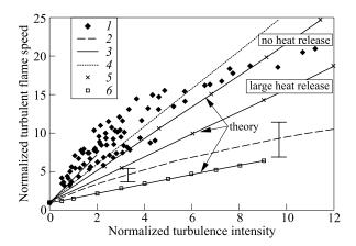
**Figure 15.4** A comparison of turbulent flame speeds measured in the TC apparatus with theoretical predictions and measurements by earlier investigators using other types of burners: 1 — TC results, 2 — Abdel-Gayed *et al.* [3], 3 — Chang and Shepherd [1], 4 — Bedat and Cheng [2], 5 — Anand and Pope [15], and 6 — Yakhot [16]
