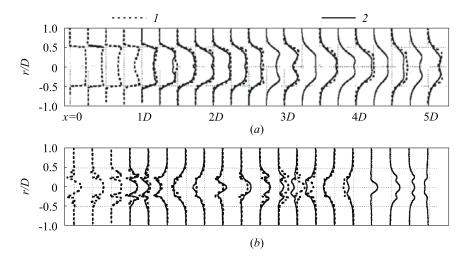
Figure 29.11 Comparison of pressure measurements in the near field of the natural (1) and excited (2) jets. Case 1: (a) total pressure profiles, and (b) static pressure profiles
