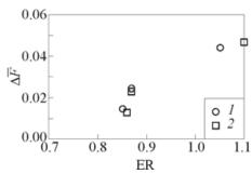
Figure 23.9 Comparison of normalized combustion induced pressure—area integral for fin-pylons with elliptic (1) and round (2) nozzles
