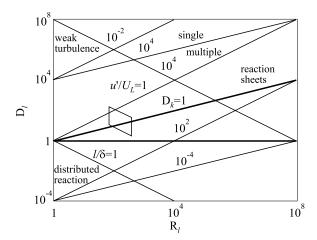
Figure 15.5 A Damköhler–Reynolds number plot revealing the turbulent combustion regimes characterizing flame propagation in the TC apparatus, identified by the region enclosed by the parallelogram
