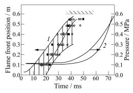
Figure 14.5 Comparison between experimental and theoretical results for turbulent flame front position and pressure—time line. Cornstarch with air at  $\rho_{av} = 0.22 \text{ kg/m}^3$
