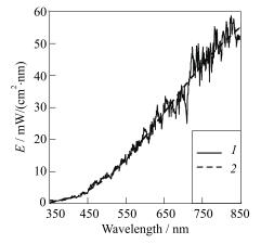
**Figure 8.2** Typical measured hemispherical emissive power distribution for the  $O_2/Ar$  oxidizer test. 1 — Port 7 Data, 2 — Fit: T = 2887 K, EM = 0.46
