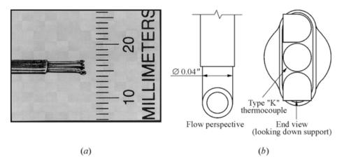
Figure 17.8 Magnified views of the Low-Profile Vectoring Velocity—Temperature probe used to capture the mass flow rate of reactants leaving the CSC
