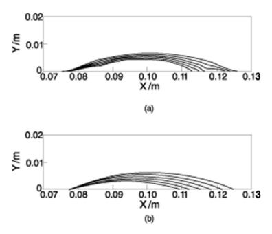
**Figure 5.6** Computed (a) and experimentally estimated (b) shape of the solid–gas interface at selected time instants. Curves from top to bottom correspond to t = 0.0, 2.5, 5.0, 7.5, 10.0, and 12.5 s
