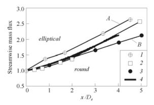
Figure 13.1 Near-field entrainment measurements in noncircular jets based on experimental and computational studies [16]. Subsonic regimes. Experiments: 1—elliptic [37]; 2— square [16]; 3— round [38]. Simulations: 4— square [16]. A:  $(D_e/Q_0)(dQ/dx) \sim 0.36$ ;  $B: \sim 0.24$
