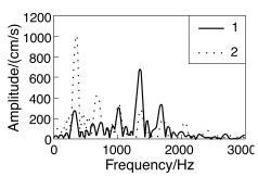
**Figure 7.8** Fourier spectrum of radial velocity fluctuations in the shear layer for unseeded flow and fully developed flow with microexploding droplets: 1 — no particles; 2 — particles
