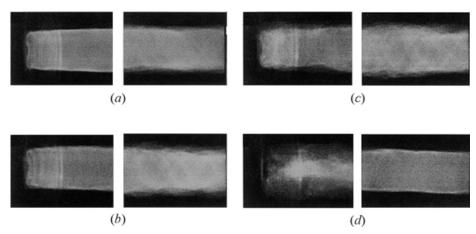
**Figure 17.4** Images of the CSC flame at the "rear" (left side of figure) and "front" (right side of figure) with rear mass fractions of 10% (a), 20% (b), 30% (c), and 40% (d) of the total mass flow delivered to the burner. Each image extends 7.5 cm axially
