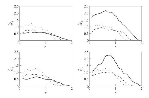
**Figure 11.4** Radial distributions of the RMS of the fluctuating vorticity components at different times for the unheated (left column) and heated (right column) jet. The times are: t = 25 (dotted curve), t = 30 (dashed curve), and t = 35 (solid curve)
