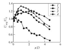
**Figure 20.5** Average centerline velocity vs. axial distance for configuration 1. No forcing: 1—no swirl; 2—high swirl. High forcing: 3—no swirl; and 4—high swirl
