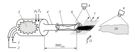
**Figure 29.3** Experimental setup and instrumentation: 1 — fuel; 2 — oxidizer,  $N_2$ , seed-particles; 3 — plenum chamber; 4 — flow straightener; 5 — c/d nozzle ( $D_{\rm throat} = 19.0 \, {\rm mm}$ ,  $D_{\rm exit} = 24.7 \, {\rm mm}$ ); 6 — cavity; 7 — laser sheet; 8 — Mie-scattering collection device; 9 — CCD; 10 — afterburning flame; and 11 — microphone
