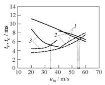
Figure 12.9 To the determination of the limiting inlet velocity  $u_{in}$  for the stabilized combustion of the stoichiometric methane—air mixture in the combustor with open-edge V-gutter flame holders. Solid curves correspond to the calculated residence time  $t_r$ . Dashed curves correspond to the calculated reaction time  $t_c$ . Flame holders with H=10 cm (1), 5 cm (2), and 2 cm (3). Conditions are similar to those in Figs. 12.6 and 12.7
