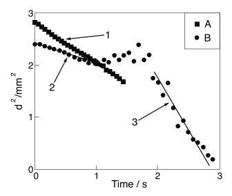
**Figure 5.3** Burning rates of pure JP-10 (A) and solution of JP-10 with 18% MPCU (B). The burning rate for the pure fuel is  $0.757 \text{ mm}^2/\text{s}$  (1). The solution vaporization rate is  $0.409 \text{ mm}^2/\text{s}$  (2), and combustion proceeds with a rate of  $1.971 \text{ mm}^2/\text{s}$  (3)
