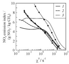
Figure 25.11 Comparison between the predicted net emission index (including all mechanisms) using RRA and numerical calculations for atmospheres: 1-1.0 bar, 300 K; 2-2.0 bar, 300 K; and 3-1.0 bar, 500 K. Curves with symbols represent numerical computations with the starting mechanism; curves without symbols represent the RRA analysis
