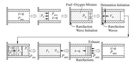
Figure 30.2 Schematic of PDE operation [9]
