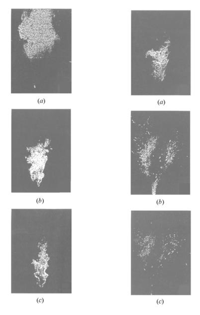
**Figure 16.1** Observed features of spray flames with three different atomization gases, (a) steam at 195 °C, (b) preheated air at 185 °C, and (c) normal air at 25 °C
