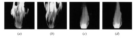
**Figure 20.4** Flame structure. No forcing: (a)  $N_S = 0.3$ ; (b)  $N_S = 0$ . High forcing: (c)  $N_S = 0.3$ ; (d)  $N_S = 0$
