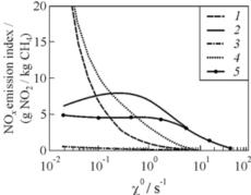
Figure 25.9 The relative contributions of the thermal  $E_T$  (1), prompt  $E_P$ (2), and nitrous oxide  $E_N$  (3) mechanisms as well as reburn  $E_R$  (4) to the emission index and the net emission index found from Eq. (25.2) (symbols 5 —  $E_{NO_x}$ ) as predicted by RRA analysis for methaneair diffusion flames at p = 1 bar and oxidizer and fuel stream temperatures of  $T_F = T_O = 300 \text{ K}$
