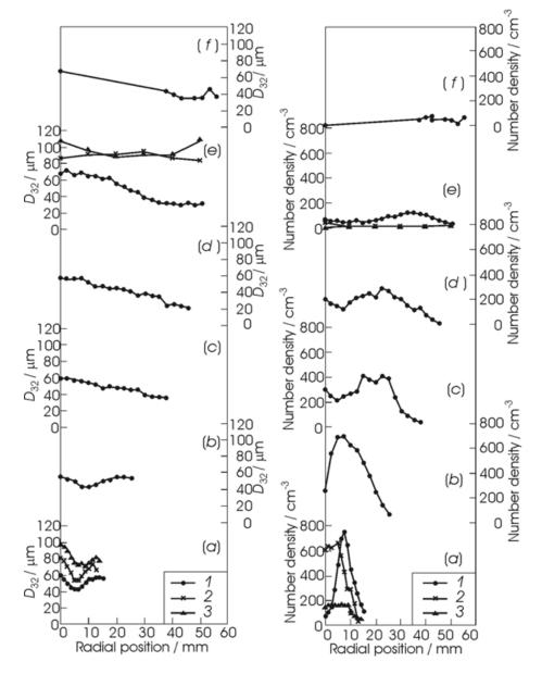
Figure 16.3 Variation of Sauter mean diameter  $(D_{32})$  with radial and axial positions for different atomization gases: 1 — steam; 2 — preheated air; 3 — normal air. (a) z = 10 mm, (b) 20, (c) 30, (d) 40, (e) 50, and (f) 60 mm
