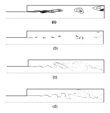
**Figure 7.2** Instantaneous visualization of vorticity contours (a), and locations of 1  $\mu$ m (b), 15  $\mu$ m (c), and 30  $\mu$ m (d) diameter particles
