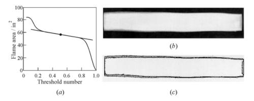
**Figure 17.7** (a) Cylindrical flame sheet area as a function of gray scale threshold; (b) corresponding flame image; and (c) image contours at threshold values of 0.34, 0.54, and 0.69
