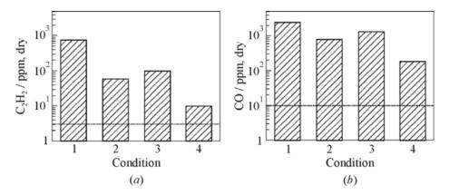
Figure 24.13 Measured  $C_2H_4$  (a) and CO (b) concentrations in exhaust of the 50-kilowatt combustor at China Lake using extractive sampling of gases from port 3 at four representative flow conditions: 1 — no forcing; 2 — primary air forcing; 3 — poor phase angle; and 4 — optimum phase angle. Detection limits indicated by horizontal dashed lines
