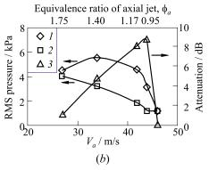
**Figure 19.8** Influence of velocity of oscillated jet,  $V_a$ , on control effectiveness; flow arrangement with swirl; Sw = 1.35;  $U_m$  = 17 m/s; Re<sub>s</sub> = 56,000; average velocity of axial jet,  $U_a$  = 42 m/s; 5% of total fuel oscillated; (a)  $\phi_0$  = 0.63; (b)  $\phi_0$  = 0.76; 1 — without control; 2 — with control; and 3 — attenuation
