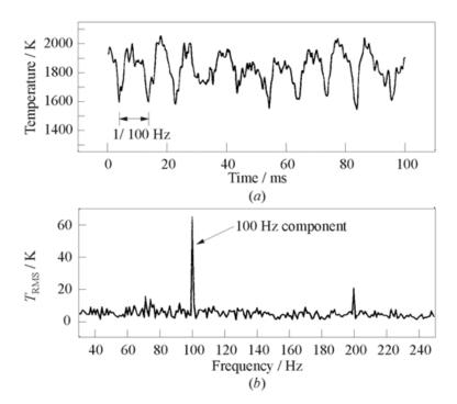
**Figure 24.4** Measurements of gas temperature recorded at 3-kilohertz rate at x/d=2 in the 5-kilowatt combustor (a) and the power spectral density (1-hertz resolution) of a 1-second history of the temperature measurements (b). Steady parameters:  $\phi=0.75$ ,  $f_0=100~{\rm Hz}$ ,  $A_{\rm air}=25~{\rm W}$ , and  $\theta_{\rm fuel}=200^{\circ}$
