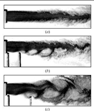
Figure 29.4 Instantaneous planar Mie-scattering images of fully expanded Mach 2 jets: (a) natural unexcited jets; (b) and (c) excited jets using flow-induced cavity resonance
