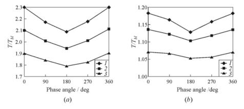
**Figure 20.8** Centerline temperature vs. phase angle,  $N_S = 0$  (configuration 1): (a) r/R = 0; (b) 0.67. 1 - x/D = 0.16; 2 - 0.34; and 3 - 0.67
