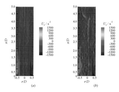
**Figure 18.6** Time-averaged strain  $U_r$  and velocity field (a) and instantaneous strain and velocity field (b) of the premixed flame for  $-U_2/U_1 = 0.0$ . The scale of the velocity vector length is 3.6 m/s per 1 mm
