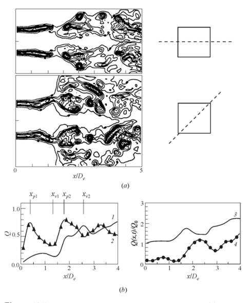
Figure 13.5 Unsteady nonpremixed combustion and fluid dynamics: (a) contours of the vorticity magnitude  $\Omega$  in planes indicated to the right; (b) cross-sectional averaged measures of instantaneous chemical product and product formation (left frame), instantaneous unconstrained and vorticity-bearing ( $\Omega > 5\%$  peak-value) streamwise mass flux Q (right frame). 1 — product, 2 — instantaneous production, 3 —  $\Omega_0 = 0$ , and 4 —  $\Omega_0/\Omega_{\rm peak} = 0.05$
