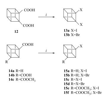
**Figure 2.19** Synthesis of substituted cubanes. Reagents: i, PhI(OAc)<sub>2</sub>, I<sub>2</sub> or Br<sub>2</sub>, benzene, reflux
