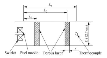
Figure 28.1 Combustor test section
