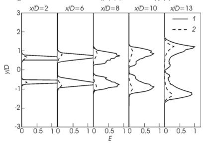
Figure 10.10 Profiles of nondimensional emission source term with large-scale turbulence–radiation interactions accounted for (1)  $\langle E \rangle$  and without them (2)  $E(\langle \widetilde{T} \rangle, \langle \overline{\kappa}_P \rangle)$
