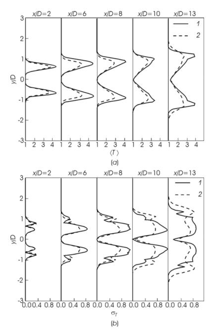
**Figure 10.4** Transverse profiles of (a) mean and (b) RMS nondimensional temperature at five axial locations without (1) and with (2) radiation
