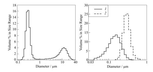
Figure 8.6 Particle size distribution for combustion products collected during H<sub>2</sub>O oxidizer test
