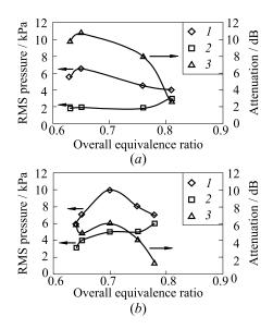
**Figure 19.10** Influence of heat release on control effectiveness; flow arrangement with swirl; Sw = 1.35; 5% of total fuel oscillated (a)  $\operatorname{Re}_m = 35,000$ ,  $U_m = 17$  m/s,  $U_a = 42$  m/s; (b)  $\operatorname{Re}_s = 70,000$ ,  $U_m = 34$  m/s,  $U_a = 84$  m/s; I—without control; I—with control control; I—with control co
