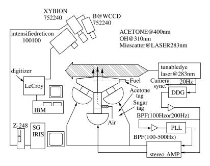
Figure 6.1 Apparatus diagram
