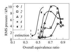
Figure 19.7 Influence of swirl on antinodal RMS pressure fluctuation; flow arrangement with swirl; bulk mean axial velocity of main flow in swirler,  $U_m = 17$  m/s, Reynolds number in swirler (for isothermal conditions),  $\text{Re}_s = U_m D/\nu = 56,000; 1 - \text{Sw} = 0.6; 2 - 1.35; 3 - 1.8; 4 - 2.4; and 5 - 3.75$
