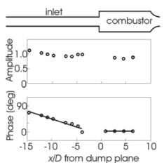
Figure 21.8 Instability mode shape for Case 1A
