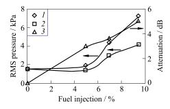
Figure 19.11 Control of oscillations by oscillation of fuel in the main flow; flow arrangement with swirl; Sw = 0.60;  $U_m = 17 \text{ m/s}$ ; Re<sub>s</sub> = 56,000;  $U_a = 60 \text{ m/s}$ ;  $\phi_t = \phi_r = \phi_p = 0.73$ ; I — without control; 2 — with control; and 3 — attenuation
