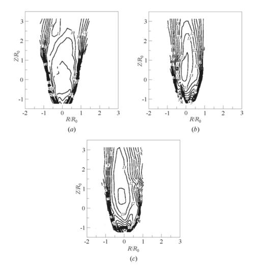
**Figure 20.13** Temperature contours for different flow conditions (configuration 3): (a)  $Q_s = 8.8$  scfm;  $Q_p = 0.0$  scfm; (b)  $Q_s = 5.0$  scfm;  $Q_p = 3.8$  scfm; and (c)  $Q_s = 8.8$  scfm;  $Q_p = 3.8$  scfm. 1 - 0 °C; 2 - 100; 3 - 200; 4 - 300; 5 - 400; 6 - 500; 7 - 600; 8 - 700; 9 - 800; 10 - 900; 11 - 1000; 12 - 1100; 13 - 1200; 14 - 1300; and 15 - 1400 °C
