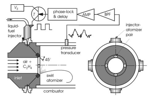
Figure 21.3 Injector set-up
