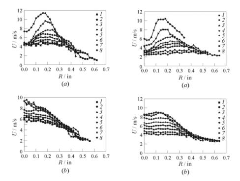
**Figure 20.10** Axial velocity measurements of droplet phase for configuration 2 without (a) and with (b) forcing: 1-z=1.5 in.; 2-1.25; 3-1.0; 4-0.875; 5-0.75; 6-0.625; 7-0.5; and 8-0.375 in.
