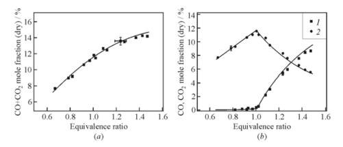
Figure 24.9 (a) Comparison of measured sum mole fractions of CO and  $CO_2$  (symbols) to calculated (curve) equilibrium values (dry basis) and (b) comparison of measured mole fractions of CO (1) and  $CO_2$  (2) to calculated (curves) equilibrium values (dry basis)
