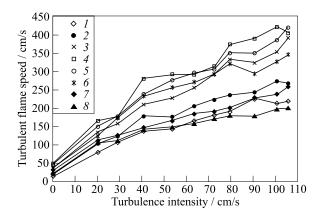
**Figure 15.3** Measured turbulent flame speeds plotted vs. measured turbulence intensities for fixed equivalence ratios from 0.8 to 1.5:  $1-\phi=0.8, 2-0.9, 3-1.0, 4-1.1, 5-1.2, 6-1.3, 7-1.4$ , and 8-1.5
