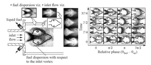
Figure 21.5 Phase-averaged fuel-droplet dispersion as a function of fuel injection timing with respect to the inlet flow vortex
