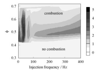
**Figure 21.7** RMS amplitude of combustor pressure oscillations at the peak instability frequency  $(10^{-2} \text{ psi})$
