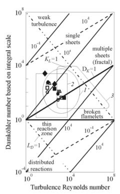
Figure 25.1 Regimes of turbulent combustion: 1 — offshore flares, 2 — spark-ignition engines, 3 — supersonic combustion,  $K_L$  — turbulent kinetic energy referred to laminar ratio of kinematic viscocity to chemical time,  $D_K$  — Damköhler number based on Kolmogorov scale,  $L_D$  — integral scale referred to thickness of laminar deflagration
