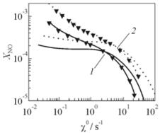
Figure 25.7 Calculated peak values of  $X_{\rm NO}$  for p=1 bar. Curves with symbols represent numerical computations; curves without symbols represent the RRA analysis:  $1 - T_O = T_F = 300 \text{ K}, 2 - 500 \text{ K}$
