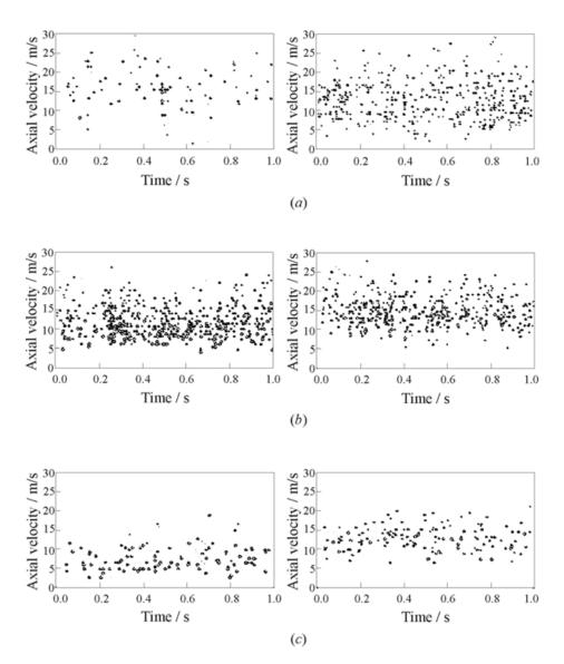
**Figure 16.7** Droplet time of arrival sequence for droplet axial velocity at z=10 mm at the spray centerline (left column) and spray boundary at r=6.4 mm (right column) for (a) steam, (b) preheated air, and (c) normal air. 1-d<10  $\mu\text{m},\ 2-d=10-30$   $\mu\text{m},\ 3-d=30$ –70  $\mu\text{m},\ \text{and}\ 4-d>70$   $\mu\text{m}$
