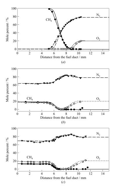
**Figure 27.1** Measurements and predictions of mole fractions of CH<sub>4</sub>, O<sub>2</sub>, and N<sub>2</sub> as a function of distance from the fuel duct for diffusion (a) and partially premixed opposed flow flames with  $\Phi_B = 2.2$  (b) and 1.42 (c),  $T_{\rm air} = 560$  K and  $T_{\rm fuel} = 321$  K,  $V_{\rm air} = 70$ , 60, and 50 cm/s,  $V_{\rm fuel} = 70$  cm/s, distance between ducts 1.5 cm
