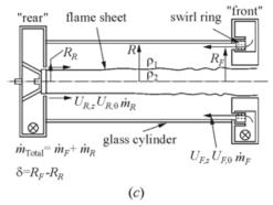
Figure 17.1 (a) Countercurrent Swirl Combustor experimental facility; (b) isometric view of the burner; and (c) cross-sectional view of the burner indicating relevant parameters
