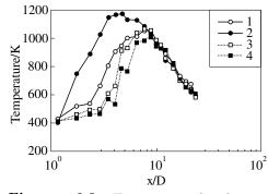
Figure 6.9 Temperature distribution along an enclosed flame centerline for different control conditions: 1 - low soot, no secondary air; 2 - low soot, with secondary air injection; 3 - low high soot, no secondary air; and 4 - low high soot, with secondary air injection
