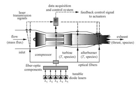
Figure 24.1 Schematic diagram for a potential application of multiplexed diodelaser sensors for measurements of gas temperature, species concentrations, velocity, mass flux, and thrust at several locations in military- and industrial-scale gas turbines (e.g., aeropropulsion, incineration, power generation applications)
