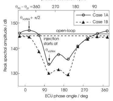
Figure 21.9 Pressure oscillation spectral amplitude as a function of injection timing. The two straight lines show the amplitude levels for uncontrolled cases
