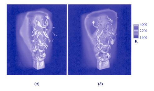
**Figure 13.7** Aspect ratio effects on the combustion of a propane–nitrogen jet with oxygen–nitrogen surroundings. Instantaneous visualizations; temperature distributions superimposed on vorticity isosurfaces [34]: (a) AR = 1; (b) AR = 2
