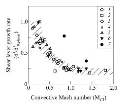
**Figure 29.9** Normalized growth rate vs. convective Mach number for natural and excited shear layers: 1 - [8]; 2 - [9]; 3 - [19]; 4 - [18]; 5 - [20]; 6 -present facility (natural); and 7 -excited with cavity acoustics
