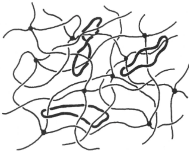
Figure 10. Topological trapping of cyclic molecules by linear chains which passed through them prior to end-linking to form a tetrafunctional network structure [44].
