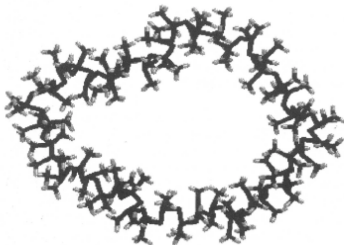
Figure 7 - Molecular model representation of a cyclic [(\text{CH}_3)_2\text{SiO}]_{50} with 100 skeletal bonds.
