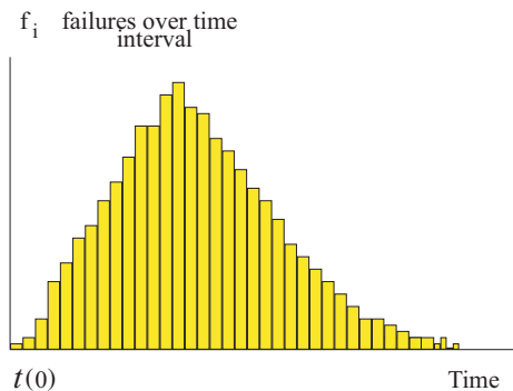
Fig. 6.2. History diagram of proportional failures against time.
