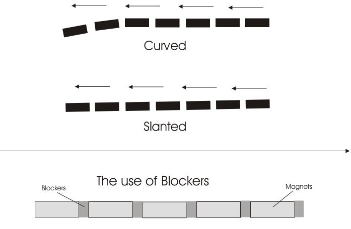
Blockers are iron or steel placed between 2 magnets, the flux field is made allot less stronger and
