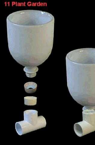
Glue 11 of the 1 inch thin wall PVC inserts and 11 of the bottle caps into seven of the 1 inch tees and four of the 1 inch corners as shown in the next slide.
