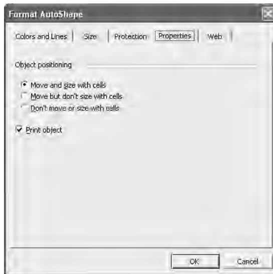
FIGURE 5-9 The Properties tab of the Format dialog box enables you to specify whether to move and resize an object along with cells and whether to print an object.
