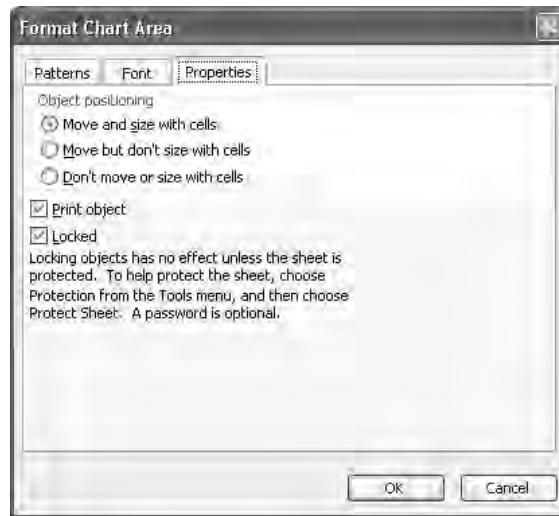
FIGURE 13-10 Use the Properties tab of the Format Chart Area dialog box to specify whether an embedded chart moves and resizes with cells, whether it prints, and whether it's locked.
