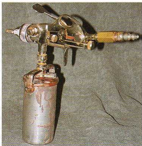
This detail gun, or jamb gun, is operated by pressing down on the lever at the top. Notice that it has a much smaller paint cup than the typical 1-quart size on a full-size production gun, making it more maneuverable for intricate, detailed areas or doorjamb.
