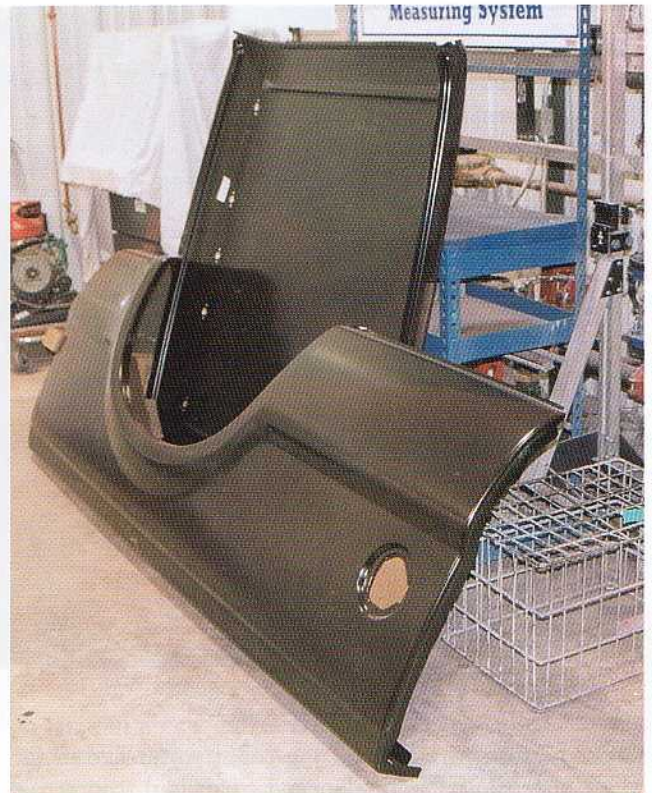
This is the bed side and roof to be installed on the Ford truck. On older trucks, it would not be an option to replace the roof, unless the old one was cut off, and a donor roof from another truck welded in place. Newer vehicles are designed with more of a component body system, allowing for easier panel replacement.
