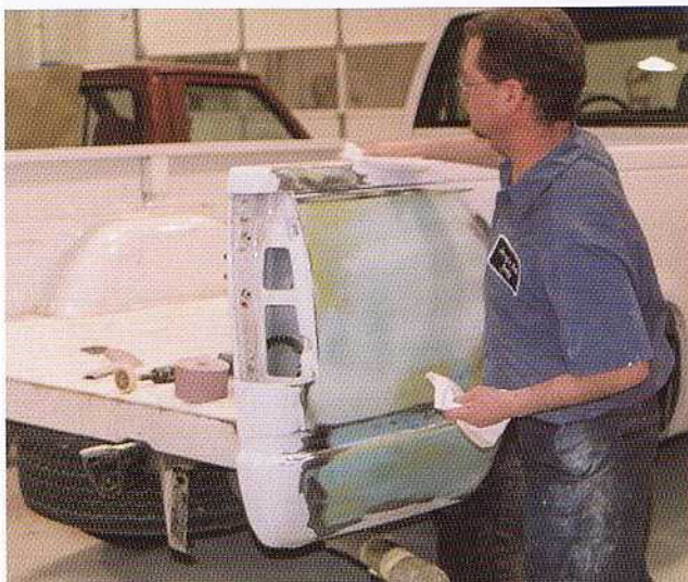
Wax and grease remover is not only preparation for the final coat of paint. It must be used prior to sanding, prior to application of body filler, and prior to application of primer-surfacer. It can be sprayed on or wiped on with a clean cloth.
