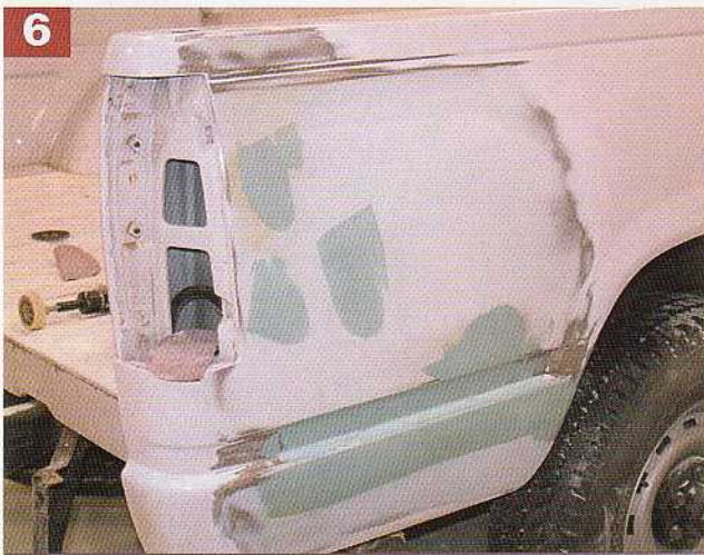
6 The bluish-green areas indicate where a thin layer of glazing filler was used to fill a slightly low spot or fill some pinholes in the body filler. The glazing filler can be sanded with 400-grit or finer sandpaper to smooth the panel to your satisfaction.
