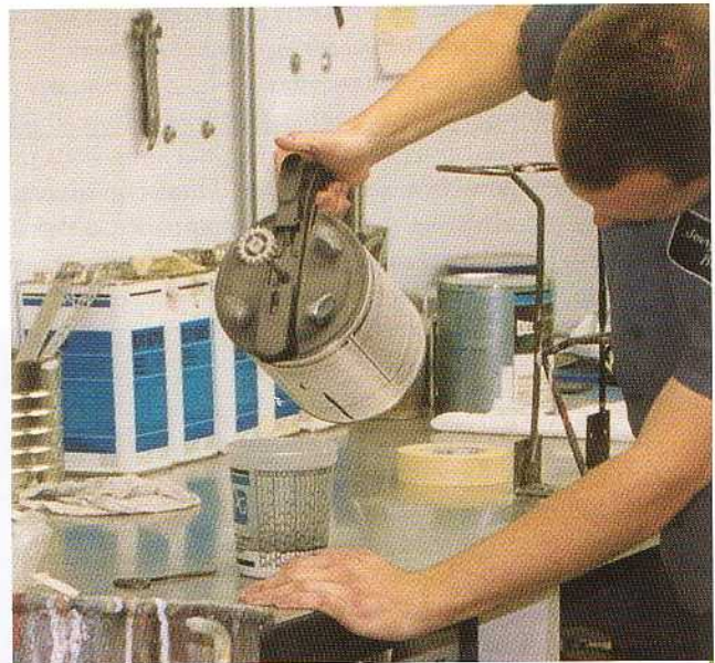
Most body shops have special dispenser caps that allow them to pour the desired amount of paint into the mixing cup. These are a convenience, but are not necessary. You will undoubtedly find that pouring from a quart can is much easier than from a full gallon can, however. Enough sealer (in this case) for the next application is poured into the mixing cup to a predetermined line on the cup. Reducer is added until the total mixture comes to the same numbered line in the next column marking the appropriate ratio.
