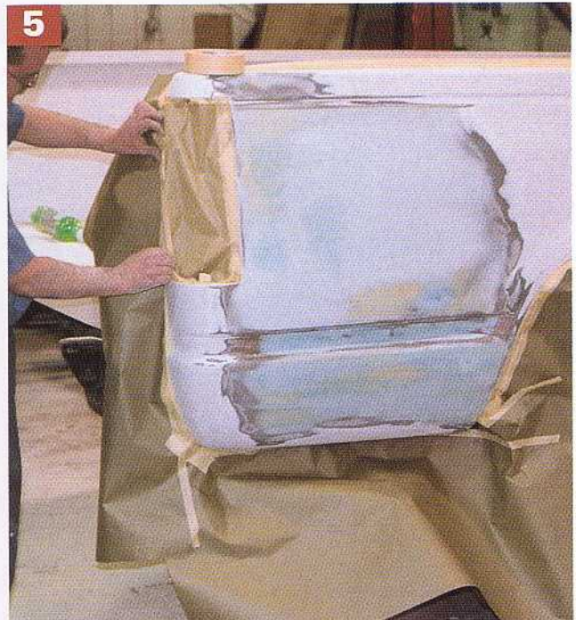
5 The taillight opening is completely masked off with narrower strips of paper.
