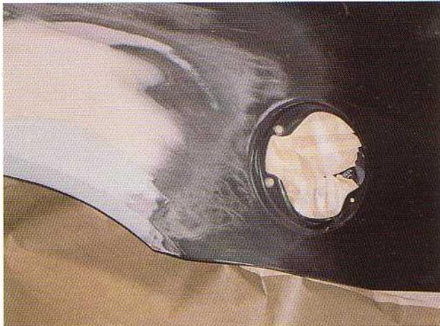
Much like the opening in the door for the door handle, the gas filler door must be masked from behind. Masking tape is now applied to the inner edge of the wheelwell to serve as an attachment point for masking paper to cover the wheel and tire. The paper is folded over as necessary to completely cover the wheel and tire, yet still be out of the way so that the wheelwell is accessible for painting.
