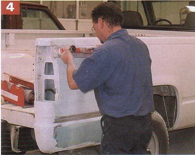
4 Using a long board or an air file will also give you a better indication of high and low spots than a smaller sanding block. The smaller sanding block will simply ride over the wavy panel, while the longer board will span the high spots and bring them down to the same level as the low spots.
