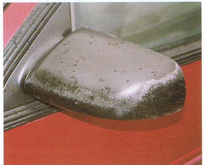
On the other hand, this rearview mirror is better suited to a spray can of touchup paint. It would be better to remove the mirror to avoid a substantial masking job. Sanding the surface with 400-grit sandpaper, cleaning it with wax and grease remover, and then spraying on a couple of thin coats of touchup would work wonders.
