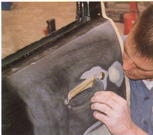
Although it is a relatively small opening, it is still necessary to close up the opening vacated by the removal of the outside door handle, as much primer-surfacer would find its way inside the car. This opening isn't being masked off from paint application, as all of the outside should be coated with primer-surfacer, and then paint. For this reason, it has to be masked from the inside. With the door open and the interior door panel removed, two pieces of wide masking tape can be overlapped to close off this opening.
