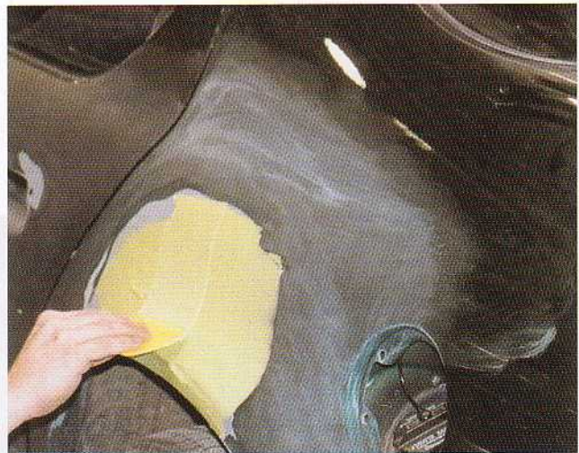
After using a slide hammer to straighten the metal to very near its original contour, the body person applies two or three thin coats of filler to match the final contour. Glazing putty can be used to fill any pinholes that remain in the sanded body filler. [see the glazed panel on page 66.]
