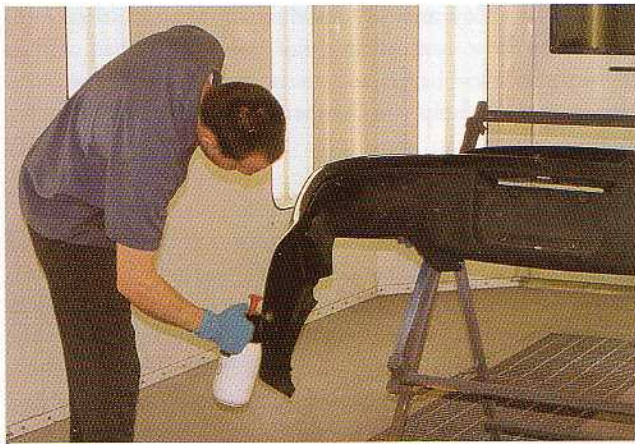
For convenience, body shops pour wax and grease remover into a spray bottle (just make sure that the bottle is labeled, as this is a clear liquid with few identifying characteristics). The wax and grease remover is sprayed, or wiped on with a clean cloth or new paper towel, and then wiped off with a second clean towel. Using anything less than a clean towel is simply defeating your purpose.
