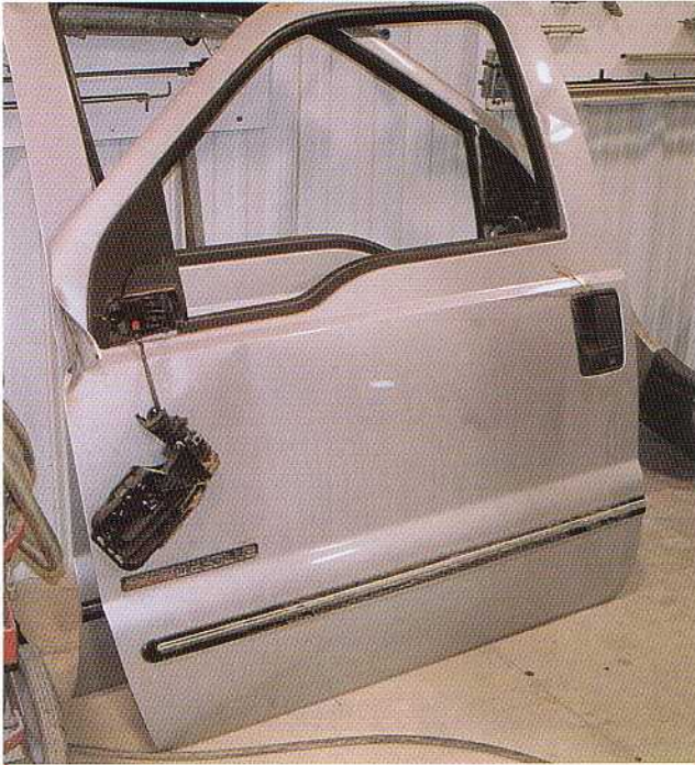
These are the two doors taken off the Ford truck in the previous photo. The left door has a major dent in its midsection, a smaller deformity in the upright behind the window, and a tear in the front of the door. Although this door could probably be saved, it would be more labor intensive. If insurance is covering the cost, a replacement door is less expensive than the time necessary to fix it or the cost of a rental car for that time. If you are paying for the parts yourself, you may choose to repair some of the affected panels.
