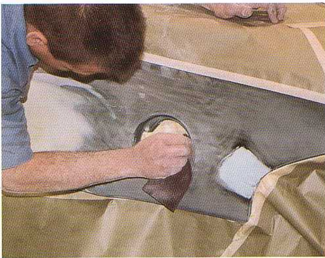
A quick double check prior to mixing primer-surfacer revealed a slight blemish in the gas filler area. It was quickly taken care of with some sandpaper. The filler to the right repaired a small ding discovered after masking began. With a little sanding, it will be ready as well.
