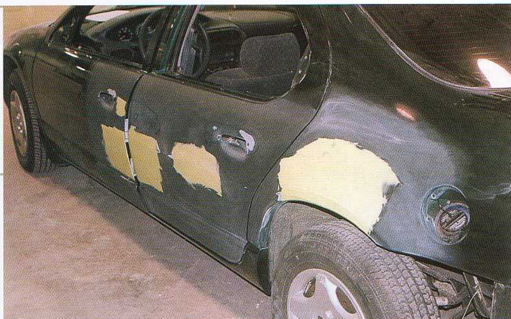
The areas of body filler show that this sedan had four small dents (two in each driver's side door) and a larger dent above the left rear wheel. If they were repainted separately, this car would have a spotted appearance so the entire side will be repainted.
