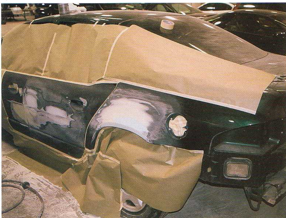
The areas of body filler show that this sedan had four small dents (two in each driver's side door) and a larger dent above the left rear wheel. If they were repainted separately, this car would have a spotted appearance so the entire side will be repainted.
