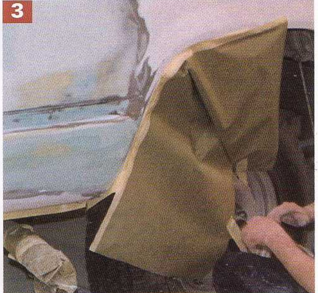
3 As the square paper is fitted around the round wheel opening, it will become necessary to fold the paper over to get it to fit properly. With tape along the inside of the lower portion of the bed side and the tailgate opening, additional masking paper is taped in place to avoid overspray on the chassis components or the inside of the bed.
