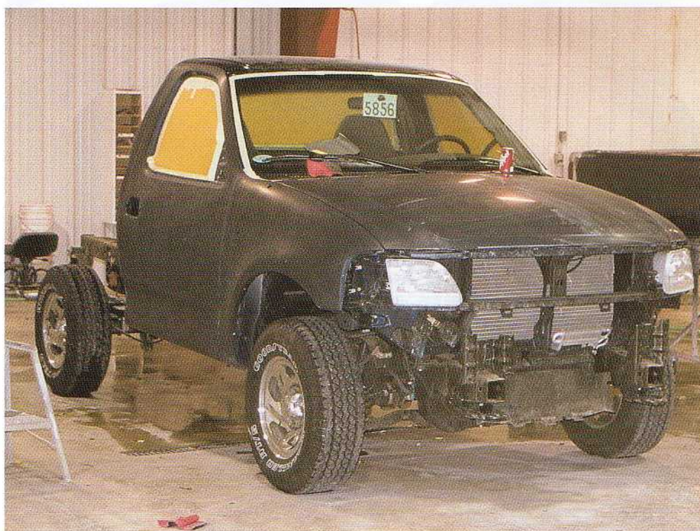
Before painting, and even prior to most of the surface preparation, the bumpers, grille, door handles, mirrors, and everything else that could be, was removed from this Ford pickup truck. The headlights will be left on in this case, as masking paper will eventually cover the entire front of the vehicle.
