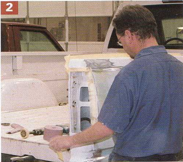
2 Masking tape is then applied to the inside edge of the taillight opening. On this particular vehicle, the taillight opening will not be painted, so it is masked off.
