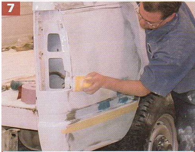
7 A normal-sized sanding block is now used to touch up the edges of the filled area. You can never sand too much. What may look great in raw body filler will quickly show any pinholes or other blemishes when you apply a coat of primer-surfacer.
