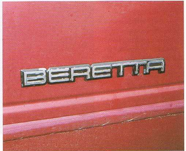
A small scratch on the sheet metal or the edges of this nameplate is the type of damage touchup paint is designed for. The small brush in the cap of a typical touchup bottle would work well to refinish this emblem, whether you remove it or not. If you had some bulk paint designed to be sprayed, you could pour some into a small container and then use a fine artist's paintbrush to touch up the emblem.
