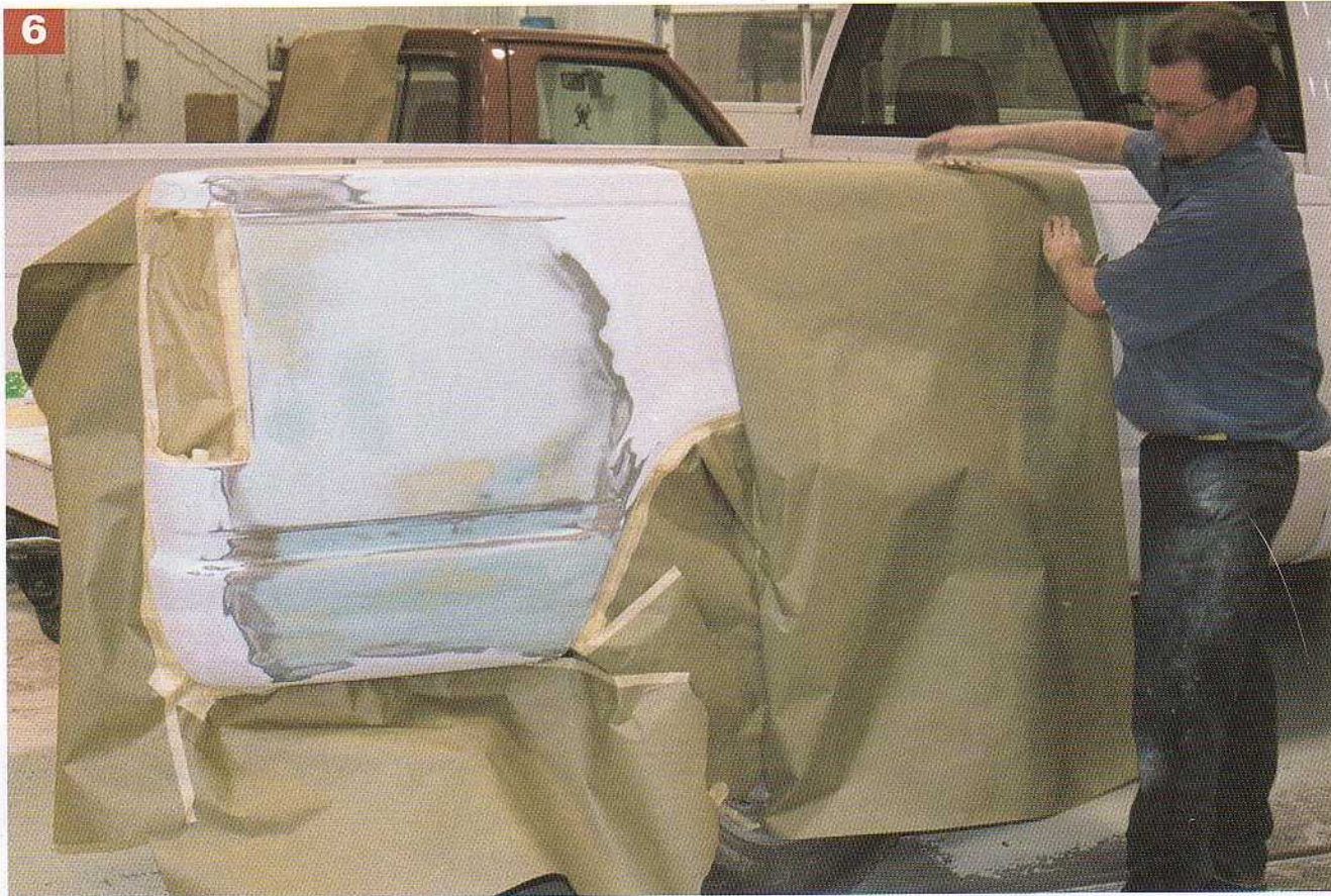
Two more wide strips of masking paper are used to cover the front half of the bedside, and another to cover the inside of the bed. Be sure to tape any seams in the masking paper.
