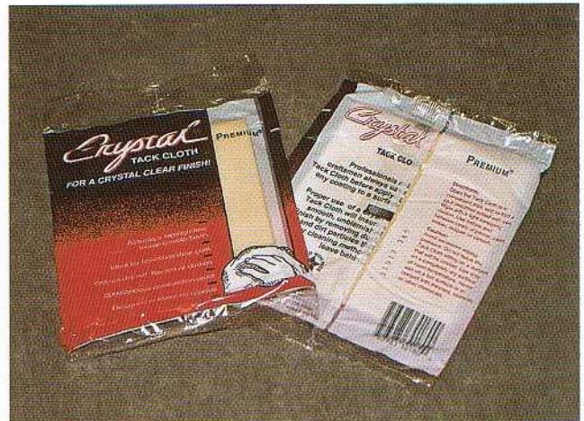
Use tack cloths to remove small particles of dust, dirt, or debris that may have been left behind by wax and grease remover. All surfaces should be cleaned with a tack cloth before you apply primer or paint. The less ideal your surroundings for spraying paint, the more you need to use a tack cloth.
