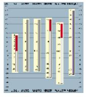
DIN and Nordic N10 variants, while Type II PPMs can commonly have either a BBC or an EBU version (see the diagram, right, for a comparison of these standards). As a rule of thumb, the scales for Type I meters generally display a considerably greater dynamic range than those of Type II, and their calibration encourages more of the system headroom to be exercised in normal use.
