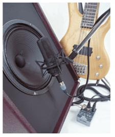
takes to travel through the air from the speaker cab to the microphone -- approximately one millisecond per foot travelled. This delay causes the two similar signals to be out of phase with each other, so that mixing them together results in comb filtering, a pattern of peaks and troughs in the frequency response which will usually weaken the combined sound.
