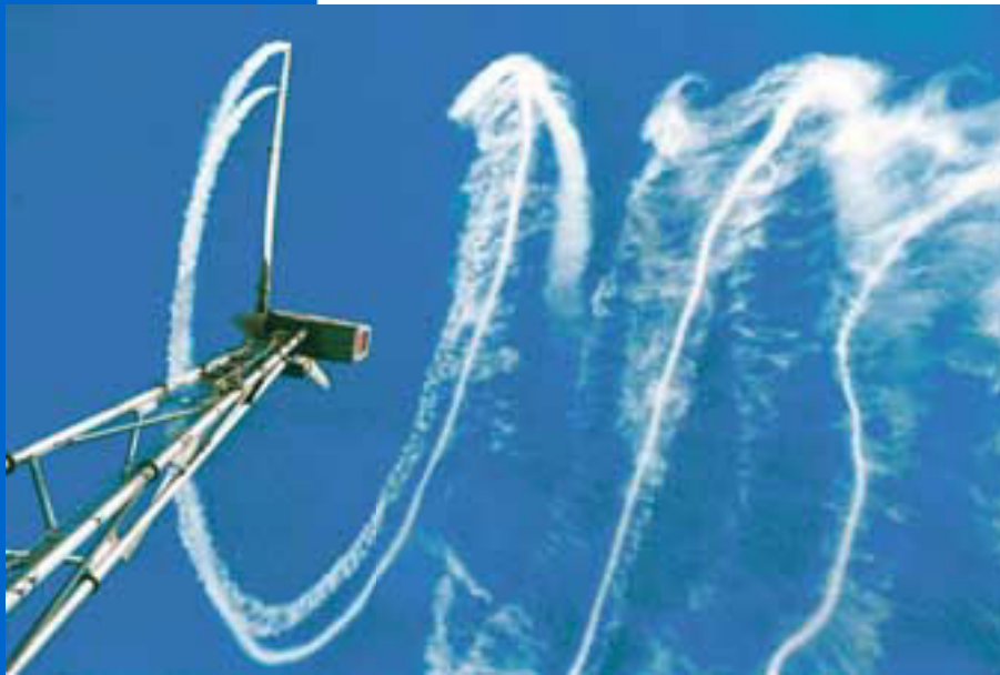
Wake effect from wind turbine Picture © Ris National Laboratory, Denmark
