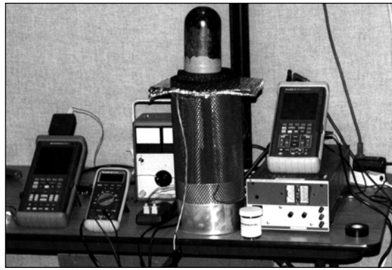
Small Case catalytic fusion cell (inside glass dewar, center) set-up for calorimetry calibration and "live" operation. Note: gas cylinder safety cap is used to secure thermal cover on dewar.
