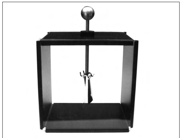
A simple, commercially available leaf electroscope.
